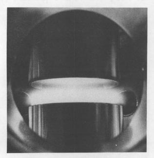
PLASMA'S characteristic glow is a result of excited gas atoms and molecules relaxing back into lower energy states. In microelectronics manufacturing, plasmas are used to etch patterns onto silicon wafers mounted between two parallel plate electrodes (seen here). As low-pressure gas is injected into the reactor, a radio-frequency voltage is applied to the electrodes, forming a gaseous mixture of ions and electrons.
